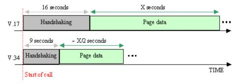
Figure 2 – Time-wise Comparison Between V.34 and V.17 Fax
