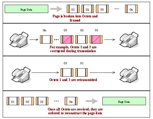
Figure 3 – ECM Enabled Fax Transmission
